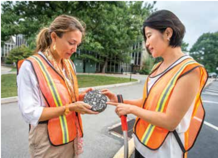
Leslie Myers McCarthy, PhD, and Seri Park, PhD, observe the aggregate gradation of an asphalt mixture after compaction.
