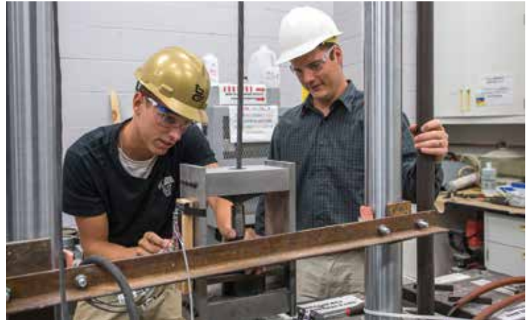
Patrick McAlpine '13 CE and Assistant Professor Eric Musselman, PhD, PE, prepare a prestressing strand for testing.
